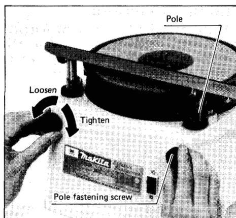
The nut for raising or lowering the pole on either side raises the pole 0.5 mm (1/32") for each graduation, when turned clockwise, and it lowers the pole, conversely, 0.5 mm (1/32") when turned counterclockwise.
