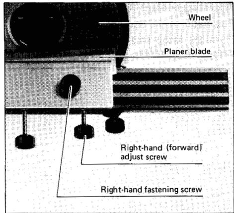
Slide the holder to the right across the sharpening platform guide. Screw in the left-hand forward adjust screw until the left upper edge of the blade contacts the grinding wheel. Now use all four fastening screws to secure the blade on the horizontal.
