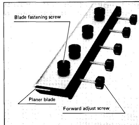
Screw in clockwise the forward adjust screw on the right until the right upper edge of the blade comes into contact with the grinding wheel. Then fully tighten the fastening screw on the far right.
